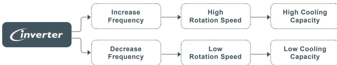
Cutting-edge inverter technology enable user to have low operating cost without losing the cooling performance. With the combination of mechanical and electronics technology, the efficiency of cooling will be magnificent coming with lower energy consumption.
